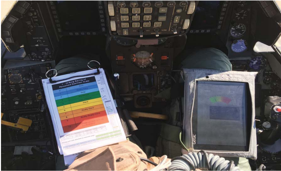
Figure 41: F-16 Internal Cockpit Perspective with Biofeedback Display
